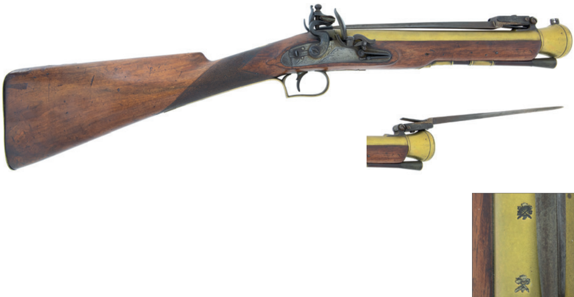
1159 Great Britain. Brass barrel flintlock blunderbuss with waterproof pan and spring bayonet. On the barrel two markings of the Birmingham Proof House. Circa 1813-1820.
