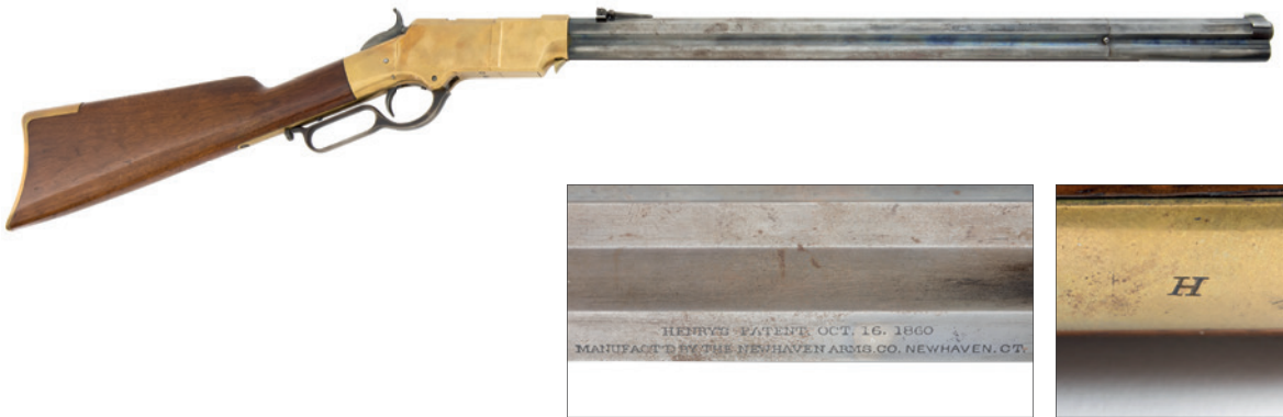
1195 United States. Henry .44 Caliber Rimfire lever-action repeating rifle. Barrel engraved 'HENRY'S PATENT. OCT. 16. 1860 MANUFACT'D BY THE NEW HAVEN ARMS.CO. NEW HAVEN. CT.'. Inspector's mark H. Serial number 2500. In good condition. Circa 1863.
